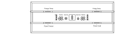
**Freezer Temp**: Indicates the current freezer temperature. **Fridge Temp**: Indicates the current fridge temperature.
