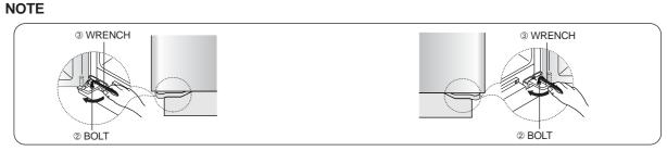
3) After adjusting the doors, turn the nut (①) turn clockwise( ) until the lower end of the bolt, then tighten the bolt again with wrench (③) to fix the nut(①).
