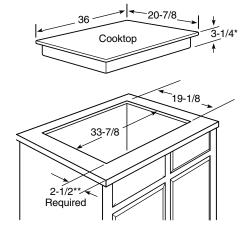
\*Depth of unit at conduit connection location (rear) is 6-1/2" on models PP980/975/950/945 and 4-5/8" on models PHP960/PP972/962/942/932/912, JP655/356/346.
