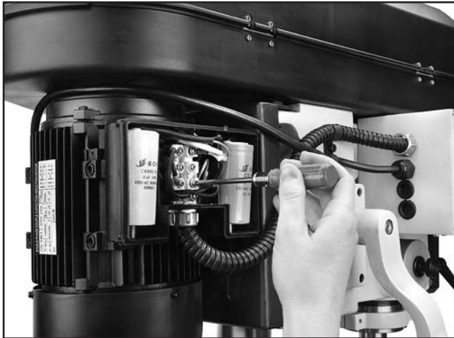
Figure 9. Changing motor jumper positions.
