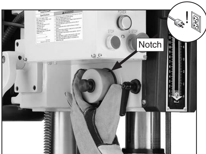
Figure 60. Adjusting spring tension.
