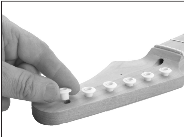
Figure 6. Installing plastic bushings on headstock.
