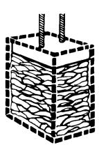
The trash in a full compactor bag will be about  $\frac{1}{4}$  the size of its original bulk.
