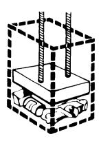
The compacting ram does not go to the drawer bottom. You will not see compacting of the first few 'badings.
