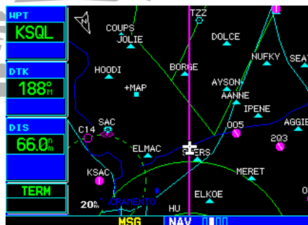
Examples of several symbols used to depict airports and nav aids on the Map page. Note the airports, Locator Outer Marker, VORTAC and Intersections.
