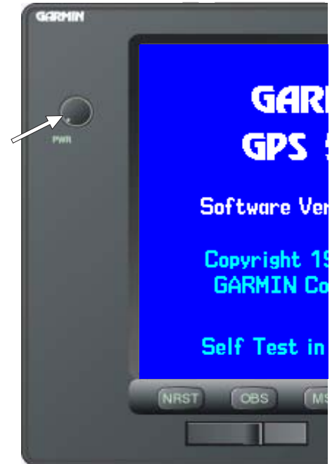
Left hand knob. Turn the unit on with the power knob on the left hand side of the unit.
