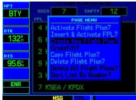
To create a new flight plan, select “Create New Flight Plan?” from the Flight Plan catalog options.
