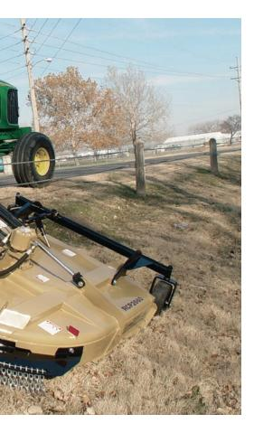
Optional gauge wheel deck allows the cutter to float over undulations without having to constantly monitor terrain conditions.
