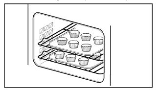
• **DO NOT** place dishes or baking trays directly on the oven base as it interferes with the oven air circulation and can lead to base burning: use the lower shelf position. However, non critical dishes may be cooked on the oven base when more space is required.
