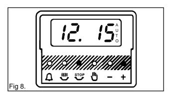
Note: When the automatic timed period starts, the oven indicator neon will cycle ON and OFF during cooking.
