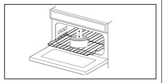
• **DO NOT** place dishes or baking trays directly onto the oven base as it becomes very hot and damage may occur.
