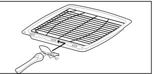
Ensure the handle is correctly located. It is not necessary to remove the grill pan handle during grilling.
