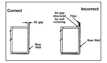
**Note:** Vapours from the oven vents may in time cause discoloration of wallcoverings behind the cooker. For ease of cleaning it may be preferable to tile behind the cooker.
