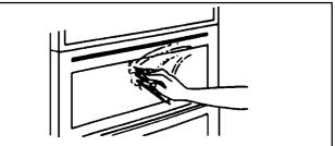
DO NOT ATTEMPT TO REMOVE ANY OF THE CONTROL KNOBS FROM THE PANEL AS THIS MAY CAUSE DAMAGE AND IS A SAFETY HAZARD.
