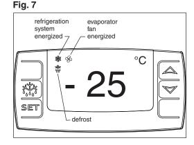
All set points have a 2 C differential. The 2 C differential means that with a -25 C set point, for example, the compressor will turn off at -25 C (-13 F) and turn on when it reaches -23 C (-9 F).
