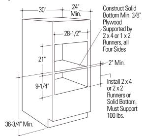
Note: Additional clearance between the cutouts may be required. Check to be sure the oven supports above the warming drawer location do not obstruct the required interior 23-1/2" depth and 9-1/4" height. See installation instructions for details.
