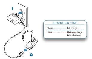
**NOTE** Never charge the battery where the temperature may fall below 0°C (32°F) or rise above 40°C (104°F) – for example, in an unattended motor vehicle. Do not charge the battery while it is unattended.
