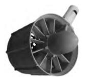
Figure 8: Motor Subassembly that Encloses the Propeller
