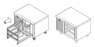
Once the drawer frame has been inserted, the drawer frame module can be installed by tighting the black front and back clamping knobs (2 of each) located on the cross rail locks and liner locks. Slide the front cross rail locks towards the center of the drawer frame module and allow the liner locks to drop down from the top of the liner. Insert the door frame module push towards the back of the unit. The entire frame assembly is now installed and ready for use.
