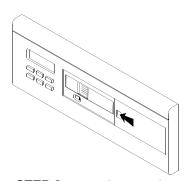
**STEP 2** - Press the magazine in until it locks in place. Slide access door closed.
