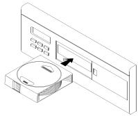
**STEP 1** - Open magazine door and gently insert the magazine oriented as shown
