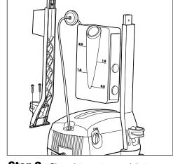
**Step 2** Place detergent reservoir between adapter brackets as shown. Attach second adapter bracket.
