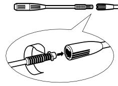
**Step 1** Install the Vario spray wand. Set the Vario spray wand to the low pressure setting (-) by turning the wand collar. The wand must be set in the low pressure (-) position to apply detergents.
