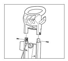
**Step 3** Attach handle onto top of adapter brackets. Press down to lock. Tighten with screws as shown.
