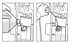
**Step 2** Fill the detergent reservoir with Cub Cadet detergent. Place the filter end of detergent suction tube into the detergent reservoir
