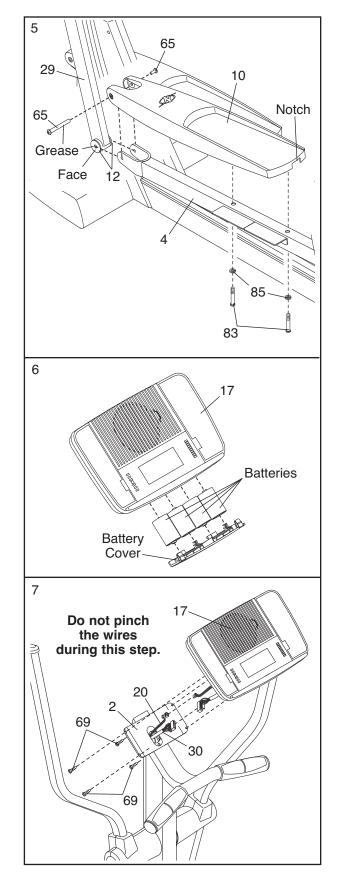
8. **Make sure that all parts of the elliptical exerciser are properly tightened.** Cover the floor beneath the elliptical exerciser to protect the floor from damage. Note: Some extra hardware may be left over.
