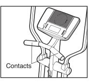
hold the handgrip pulse sensor, with your palms resting against the metal contacts. **Avoid moving your hands or gripping the contacts tightly.**
