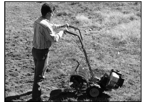
Fig. 4-4: To begin turn, lift handlebars until tines are out of ground and unit is balanced.
