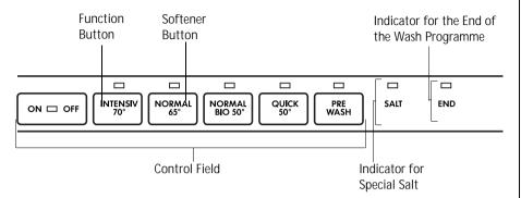
The **Control Field** comprises the On/Off switch on and the programme buttons with LED indicators.
