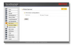
A USB printer, plugged into a USB port on the rear of your TeraStation, may be used as a *Windows Print Server* on your network by choosing *Enable* and then clicking *Apply*.
