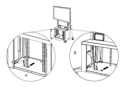
4. Straighten the rack rail, aligning the holes in the flange at the top of the rail to the pilot holes in the cabinet's top panel, and then secure the rail with two of the screws that you removed step 2.
