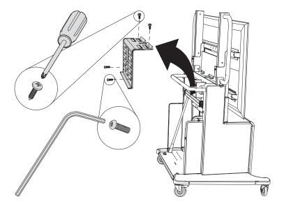
4. Remove the two installed shelves from the cabinet, and then remove the eight shelf clips.
