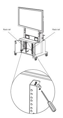
3. Lift the left rack rail at a slight angle to detach it from the base, rotate it 90° clockwise, and then insert the rail at a angle into the rack mount slots further to the left.
