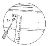
5. Repeat steps 3 and 4 for the right rack rail, except rotate the rail counter-clockwise before inserting it into the rack mount slots.
