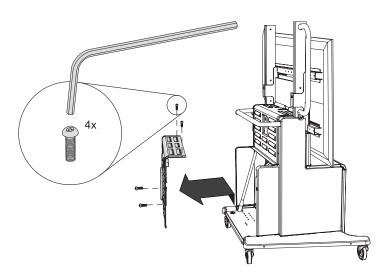
2. Remove the top two screws in the upper rear panel with a Phillips No. 2 screwdriver. Keep these screws nearby.
