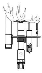
Figure 41- Correct flame pattern
