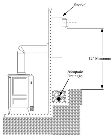
Figure 19- Snorkel Termination with Drainage Pipe
