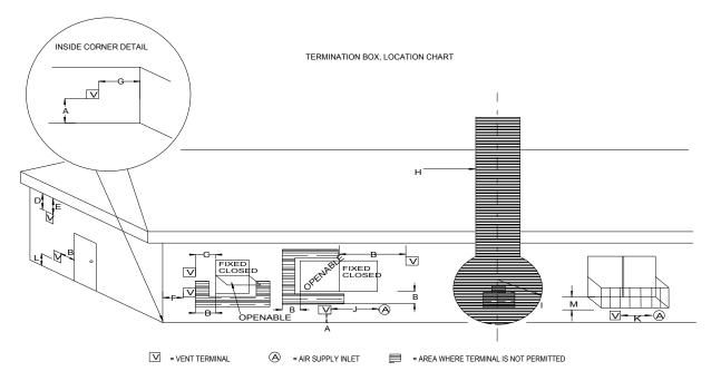
Figure 17- Minimum Clearances fo Vent Terminations
