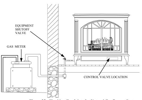
Figure 35- Checking Gas Joints for Natural Gas Burner System
