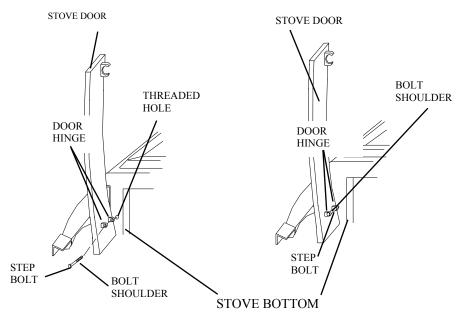
Figure 10-Attaching Lower Stove Door Panel
