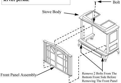
Figure 37- Removing Front Panel from Stove
