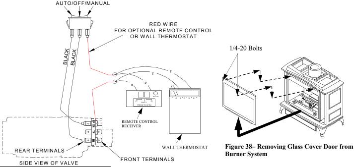
WARNING: Do not connect this thermostat to a power source. Electrical shock and/or fire hazard will occur.
