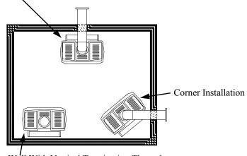
On Wall With Vertical Termination Through Ceiling
