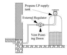
Figure 30- External Regulator with Vent Pointing Down (LP Only)
