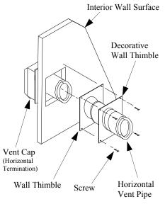
Figure 24– Connecting Vent Cap with Horizontal Vent Pipe
