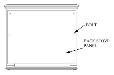
FIGURE 6 - REMOVING BACK PANEL
