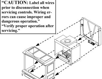
Figure 14– Installing Burner System and Blower System.
