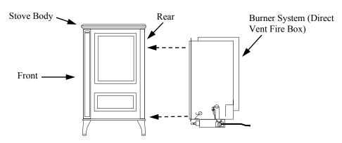
Figure 13-Installing Burner System into Cast Stove body.
