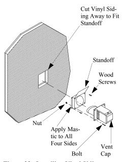
Figure 23– Installing Vinyl Siding Standoff
