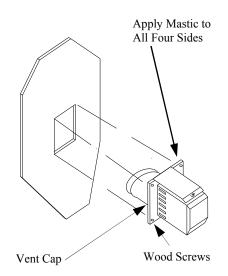
Figure 22– Installing Horizontal Vent Cap
