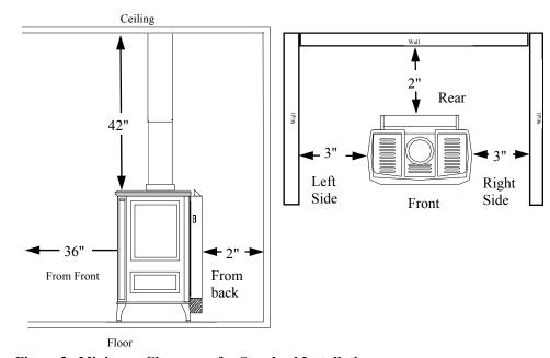
Figure 3- Minimum Clearances for Standard Installation
