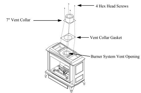
Figure 15- Installing Vent Collar
