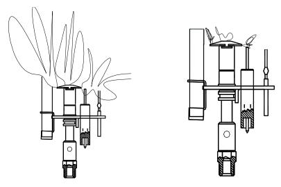
Figure 42– Incorrect flame patterns
