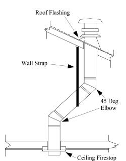
Figure 26-Offset with Wall Strap and 45 deg Elbows
