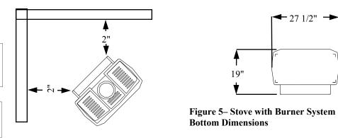
Figure 4– Minimum Clearance for Corner Installation
