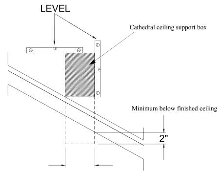
Cut hole 1/8" larger than support box when projected onto roofing
