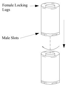
Figure 20- Rigid Vent Pipe Connections
