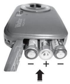
Insert 3 AAA (1.5V) batteries. Alkaline batteries recommended (not included).
