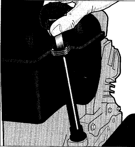
Figure 5-6: Checking the engine oil level on the 6HP Tecumseh engine on the Econo-Horse tiller.
