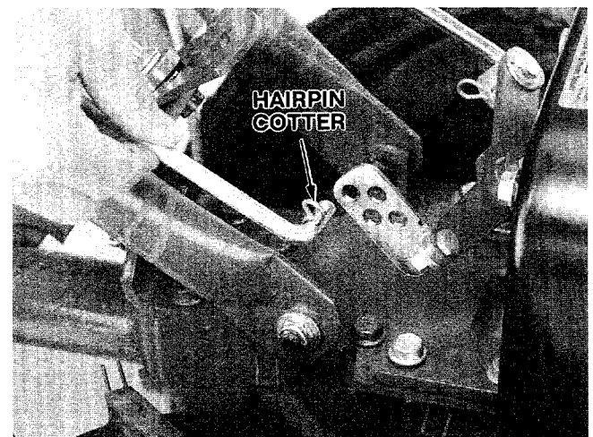
Photo 2-9: Connecting the Forward Clutch Rod.
