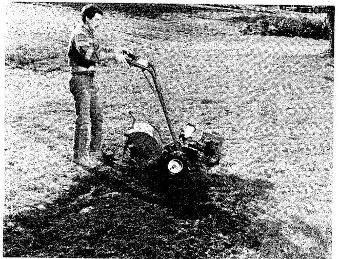
Photo 4-3: Use the wheels as a pivot point to balance the engine and tines. Push the handlebars sideways to move the tiller in the direction of the turn, and continue up the next row.
