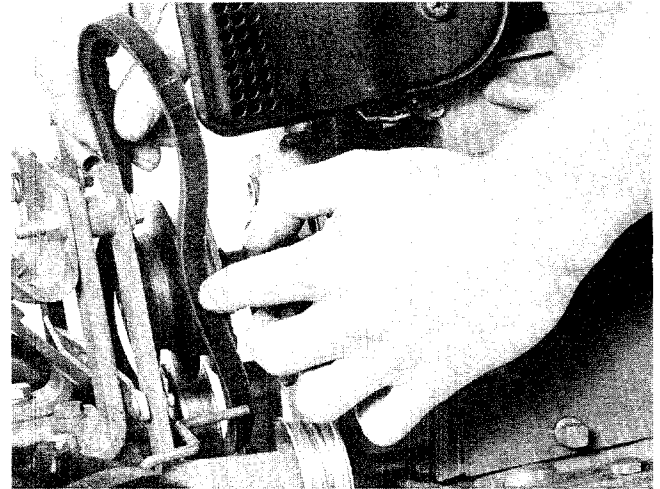
Photo 5-19: Installing the Forward Drive Belt.
