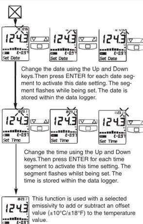
The OFFSET feature allows the temperature values for several units to be matched, correcting for the allowed temperature tolerance difference between units. The OFFSET function can also be used to increase the accuracy for a narrow temperature range.
