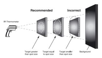
Make sure that the target is larger than the unit's spot size. The smaller the target, the closer you should be to it.
