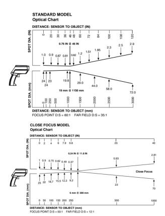
The measured spot size depends on the distance between the object you are measuring and the infrared thermometer.
