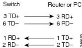
Figure 35: Identifying a Crossover Cable
