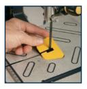
5. Loosen the blade tension knob to slacken the blade.
