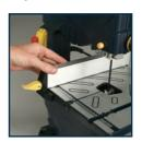
4. Attach the rip fence to the table and secure it by pushing down the rip fence locking handle (29).
