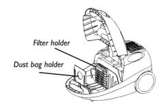
When vacuuming fine dust particles, the fine dust particles can clog the pores of the dust bag and the dust bag indicator will indicate full. If this happens the bag could appear relatively empty, however the bag will still need to be emptied to avoid strain on the motor.
