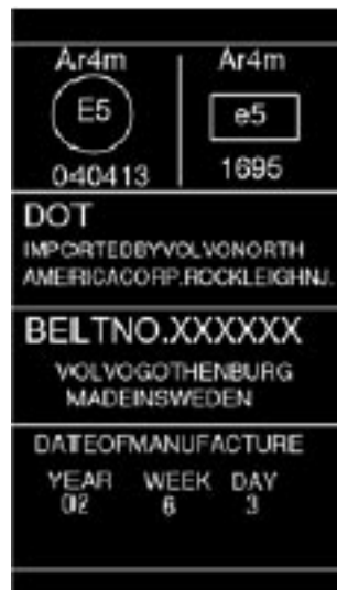
Sample label found on all seat belts with tensioners
