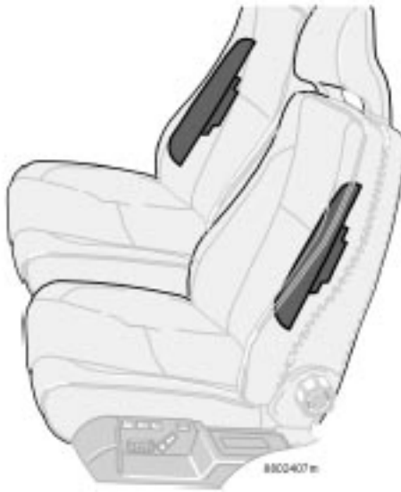
Location of the side impact (SIPS) airbag
