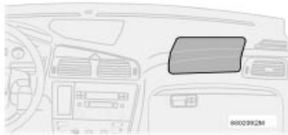
Passenger side airbag - above glove compartment
