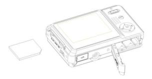
3. Push the card in until you feel it "click" into position. The top of the card should be flushed with the surface of the camera. An **SD** icon will appear on the LCD screen after you turn on your camera.
