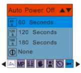
Press the Up/Down button to select a time that the camera will automatically power off if inactive.
