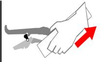
Lift the door upwards and outwards until it is free of the hinge housing
