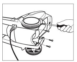
**Step 1** Attach the mobile adapter brackets to the pressure washer. Align holes on the bottom of the pressure washer as shown and tighten the 4 screws.
