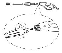
**Step 4** Slide the spray wand extension into the gun. Turn the wand collar onto the gun threads until tight.
