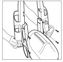
**Step 2** Spread handle sides apart and align with slotted areas of mobile adapter brackets and snap into position. Tighten the 4 screws.
