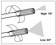
Turn the wand nozzle clockwise for high pressure. Turn counter clockwise for low pressure.
