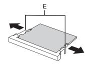
2 Carefully remove the RAM module from the slot.
