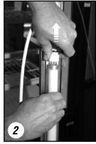
Remove bulb by gently pulling up on spring loaded lampholder.
