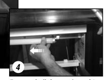
Remove bulb by gently pushing bulb into spring loaded lampholder.
