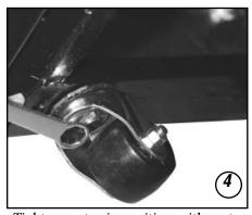
Tighten castor in position with castor wrench.
