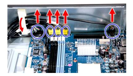
10. Remove the front I/O and card reader board bracket.
