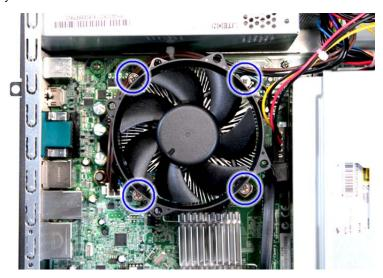
**4.** Lay down the heat sink fan assembly, in an upright position, on top of the optical drive, as shown below, then disconnect the fan cable from the mainboard.
