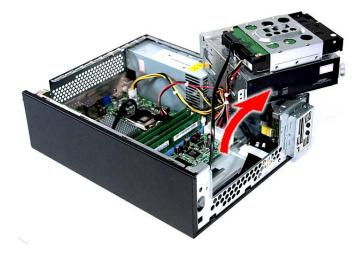
(4). Disconnect the data and power cables from the HDD.
