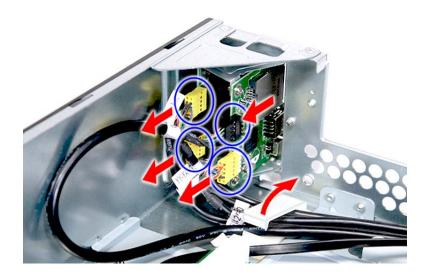
Open the cable retention clip and disconnect the other end of the USB, 1394, and audio cables from the mainboard.
