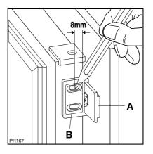
Should adjustment of the furniture door be necessary, use the clearance of slots as required.
