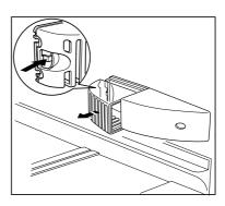
press on the rear hook and at the same time slide the cover in the direction indicated by the arrow. Unscrew the bulb and replace it with a new 25 watt bulb (available from your nearest Service Force Centre).
