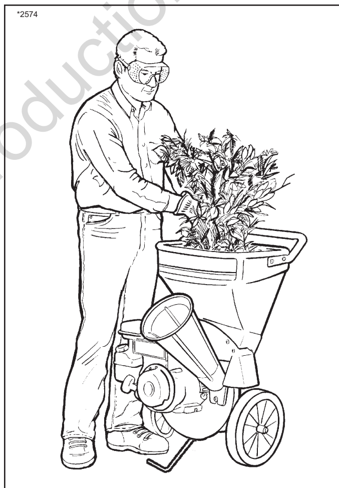
Figure 9. Properly Feeding Longer Materials for Shredding
