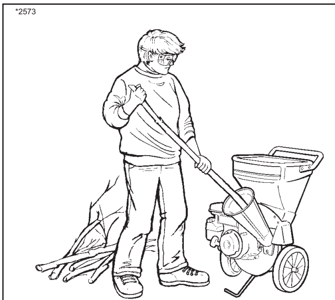
Figure 7. Proper Stance for Chipping
