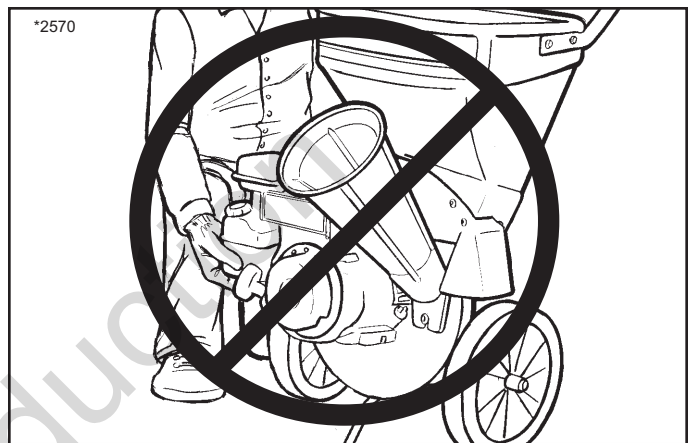
Figure 15. Improper Lifting Of Unit
