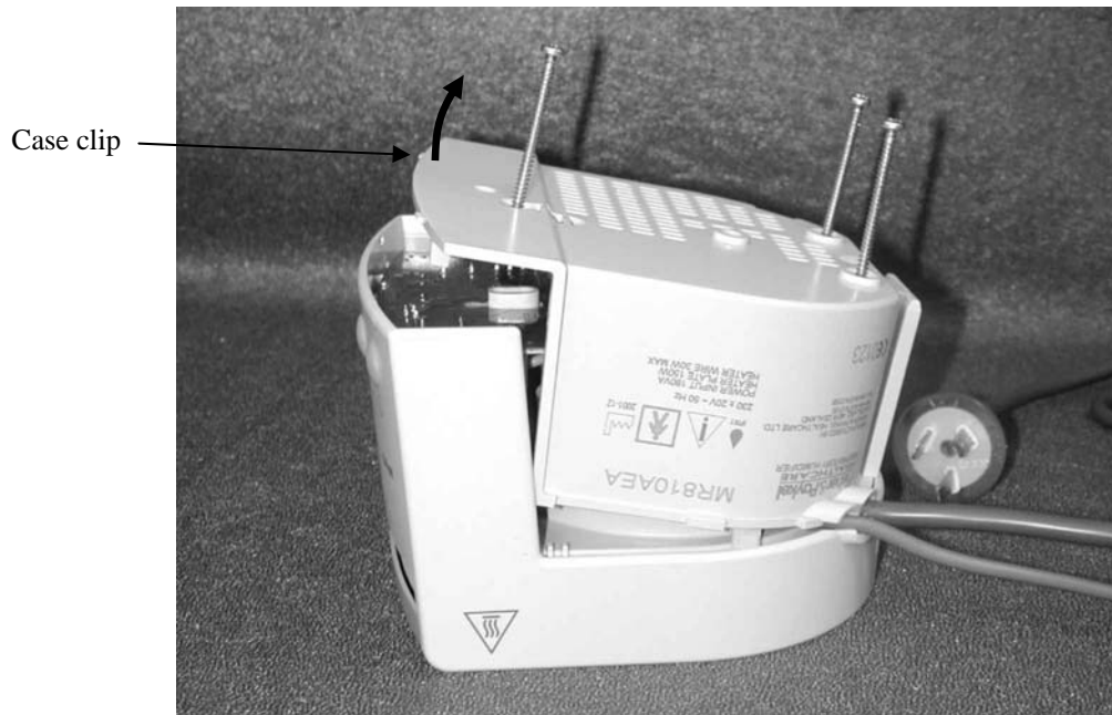
Figure 6.1: Removing the case bottom
