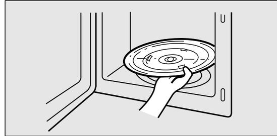
7. The roller guide and oven cavity floor should be cleaned regularly to avoid excessive noise.
