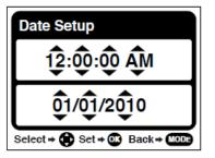
Set the Date and Time as desired by pressing the **RIGHT** and **LEFT** direction control buttons to choose the specific setting and the **UP** and **DOWN** buttons to change each setting.
