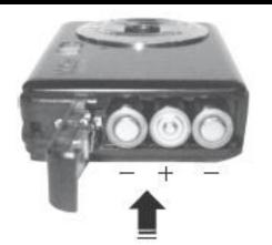
• Insert 3 x AAA (1.5V) batteries. Alkaline batteries recommended (not included).
