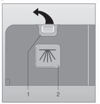
Fill the detergent dispenser with detergent. The markings are an aid to correct dosing:
