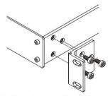
Place the ears of the machine against the rack rails, and insert the proper screws (not provided) through each of the four holes in the rack ears.
