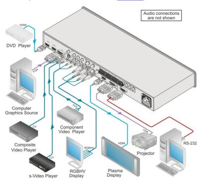
Figure 3: Connecting the VP-436N Presentation Switcher / Scaler
