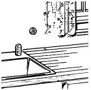
An air gap protects your dishwasher against water backing up into it if a drain clogs. The air gap is not a part of the dishwasher. It is not covered by your warranty. Not all plumbing codes require air gaps, so you may not have one.
