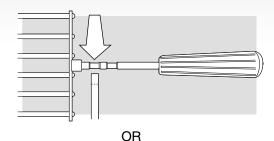
Set the Handle Shaft on the cooking box. The groove closest to the handle fits the Genesis Silver B, C, all Golds, and all Platinum gas grills. This groove should rest in the cut-out in the cooking box for the Genesis Silver B, C, all Golds, and all Platinum gas grill.
