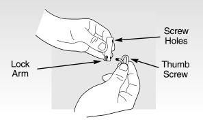
Insert middle Meat Clamp Arm into top into top of the Lock Arm as shown. Tighten top Thumb Screw to lock Meat Clamp into shaft.
