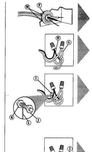
Install a U.L.-listed/CSA-certified strain relief (F) to the terminal box. Run power supply wire through strain relief. If using conduit, use a U.L.-listed/CSA-certified conduit connector. Run conduit through connector.
