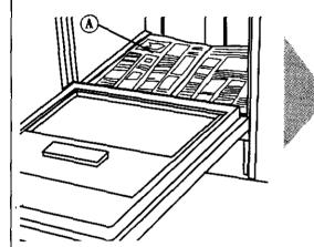
Open dishwasher door and remove all shipping materials. Remove bottom rack. Place newspaper (A) or towel over bottom of dishwasher to prevent screws from falling into pump area when securing dishwasher to countertop.
