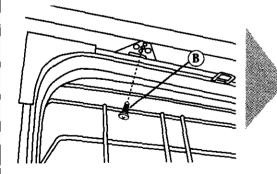
The dishwasher MUST be secured to countertop or floor to keep it from tipping when door is opened.
