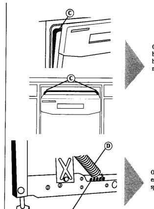
Open door about 3 inches (7.6cm) and check for equal spacing (C) between inner door and tub sides. If spacing is not equal, loosen bracket screws and shift tub. Tighten bracket screws. Remove newspaper or towel from dishwasher.
