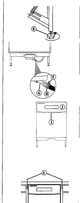
Adjust the front leveling legs (E) the number of turns listed in the chart. The dishwasher should be installed as level as possible from front to back.
