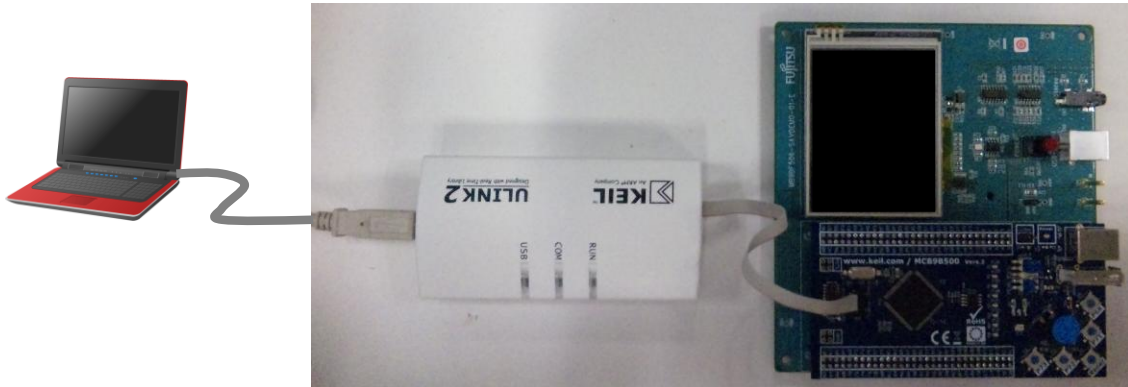
Figure 12 Equipment Connections for Exporting Program
