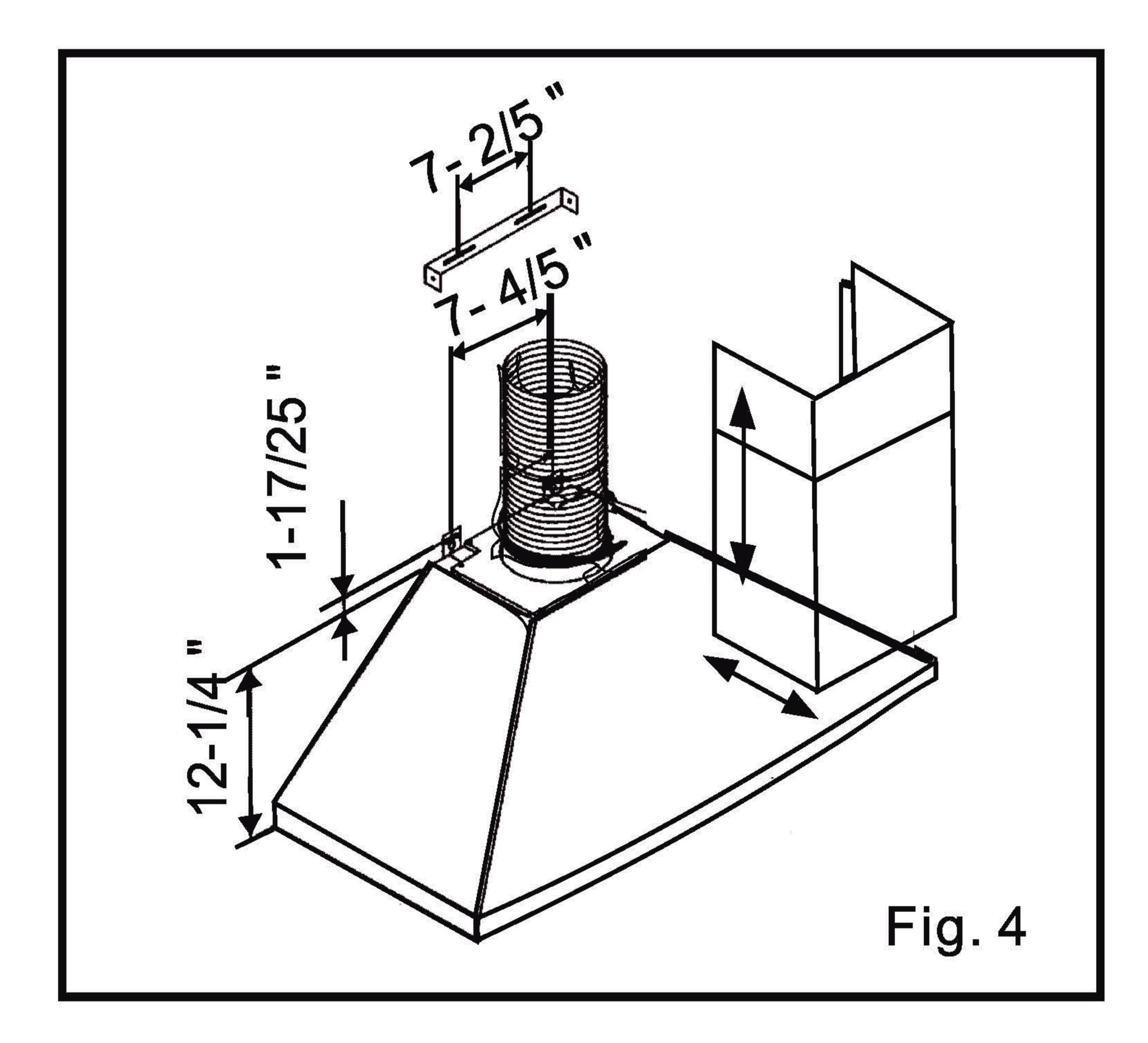
The two holes depend on cowling bracket position for adjusting.
