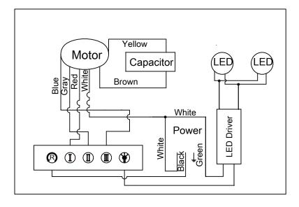
Fig.8 RA-77 Series Electrical Schematic Diagram
