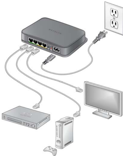
Figure 4. Connecting devices to an XAV5004 Powerline adapter
