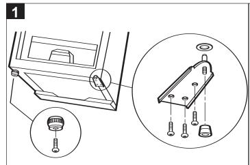
To access the lower hinge assembly, tilt back the refrigerator cabinet or lay the refrigerator on its back.
