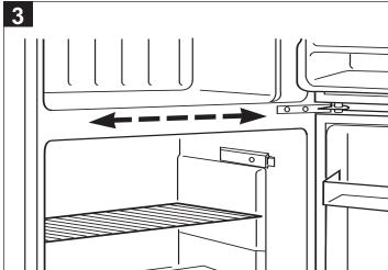
Re-install the middle Hinge assembly on the opposite side.
