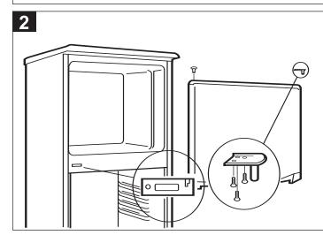
Remove the screws from the middle hinge assembly. Then remove the hinge and freezer door.
