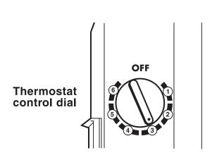
The Thermostat for the refrigerator and freezer is located at the upper right hand corner of the refrigerator compartment.
