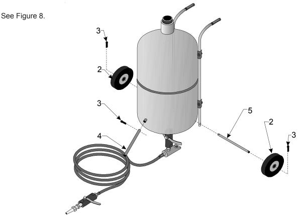
Figure 8 - Wheel and Foot Attachment
