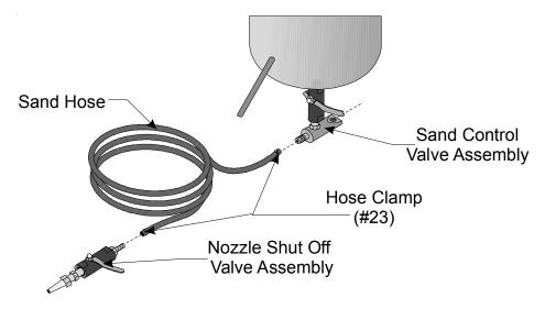
Figure 5 — Sand Control Valve / Shut Off Valve Assembly
