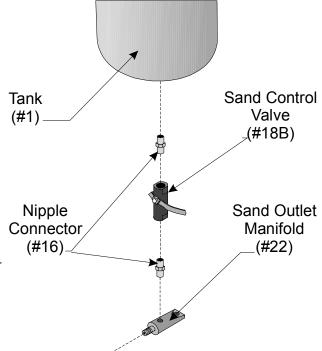
Figure 3 — Sand Control Valve Assembly
