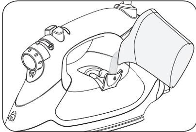
Open the Flip Funnel™ and add water to the tank with the fill cup or directly from a faucet.
