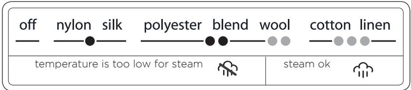
Turn the fabric selector to select a fabric setting. To use constant steam or steam burst, the temperature must be set to the wool, cotton, or linen range.
