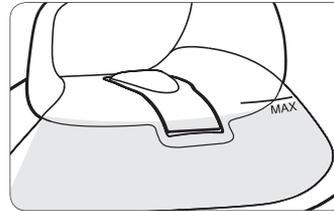
Alternatively, fill directly from a faucet holding the iron horizontally. Do not fill the tank past the MAX fill line on the side of the iron. Close the port when done.
