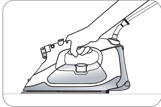
Touch the iron handle and the iron will sense your hand and lower. Let go and the iron's Lifters will automatically raise the iron above fabric.
