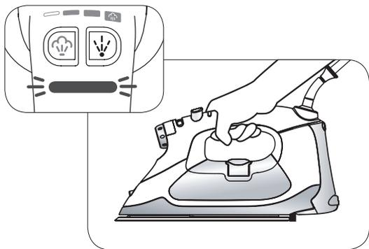
When the green light stops blinking and is constantly lit, the iron is ready for use. Touch the handle and begin.
