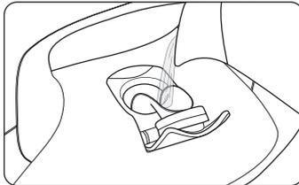
Leave the iron in a horizontal position and fill using the included fill cup. Two fill cups equal the maximum capacity of the water tank.
